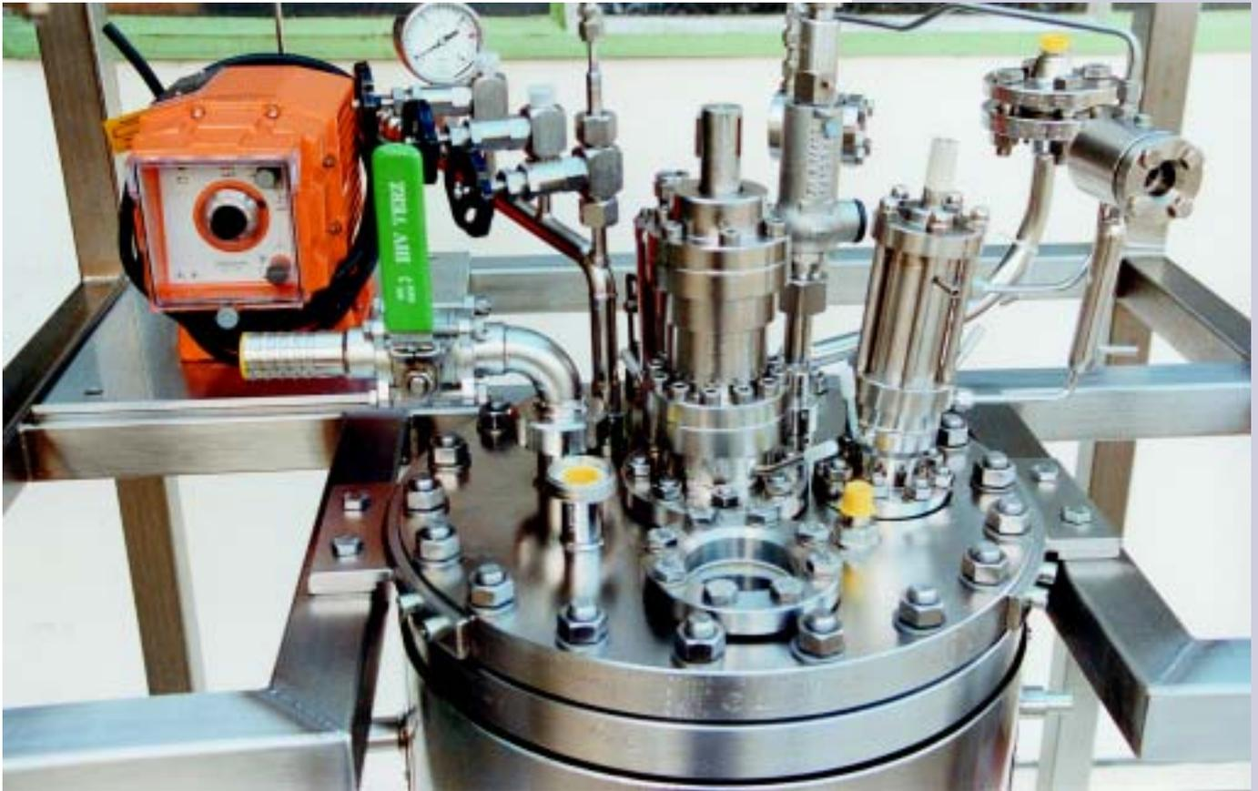
**Reaction vessel, 50 litres, in stainless steel framework**
